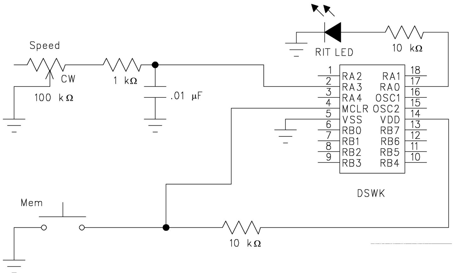
The first is pot speed control. A .01 μF polyester timing cap and a 1 kΩ resistor were supplied with the DSWK. The user will have to supply a 100 kΩ linear pot and knob to finish this mod. The user will also need to find an appropriate place to put the pot on the rig. The best position will depend on the size of the pot and the user's preference, but generally the shorter the wires to the pot, the better!
