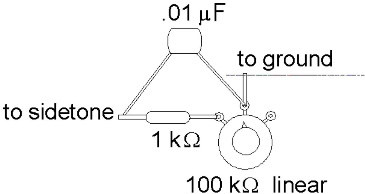
Connect the wire labeled “to sidetone” to the PIC pin 2 at the input side (facing RFC3) of C23 (DSW) or C17 (DSW-II) I was able to make this connection on the top of the circuit board by tack soldering the wire to the capacitor circuit board pad. Connect the wire labeled “to ground” to a ground point either near the pot or on the circuit board. I made this ground connection at the ground side of C101 (towards RFC3) on the DSW.
