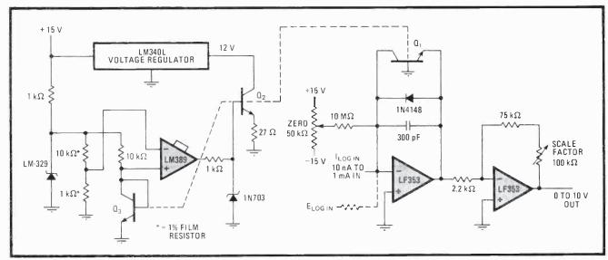
3. Holding heat. The LM389's servo loop,  $Q_2-Q_3$ , performs low-cost temperature compensation for the LF353 op amp, which is configured as a logarithmic amplifier. The chip temperature, initially determined by current through  $Q_2$ , is set with the 1-k $\Omega$ -to-10-k $\Omega$  resistive divider.
