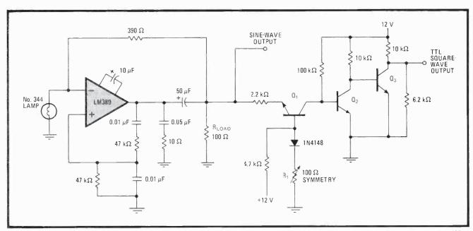
2. Sines and squares. This oscillator provides a 1-kHz sine-wave output and synchronous in-phase square waves. The amplitude-limited Wien bridge contributes to low distortion (0.2%). Single-knob calibration for synchronization is provided by potentiometer R<sub>1</sub>.
