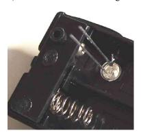
9) bend the base (center lead) of the transistor as shown:
