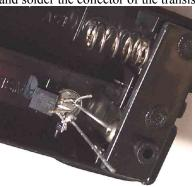
11) solder one lead of the 1.2 kohm resistor to the pre-bent center lead (base) of the transistor.
