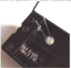
8) thread the black wire through the 1/16" hole and solder it to the short lead of the LED:
