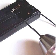
4) drill a 3/16" hole about 25/32 from the top of the battery holder, use the + symbol within the circle:
