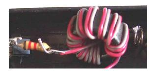
16) solder the longer toroid wire to the collector of the transistor:
