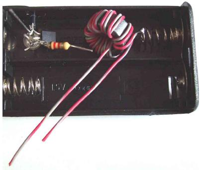
15) solder the shorter toroid wire to the 1.2 kohm resistor:
